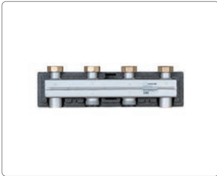
tubra®-VM St DN 25 Steel manifold, closed design for up to 5 heating circuits, DN 25, center-to-center distance 125 mm, compatible with tubra®-PGM/PGR with zinc-lamella coating WP040000 VM St DN 25
