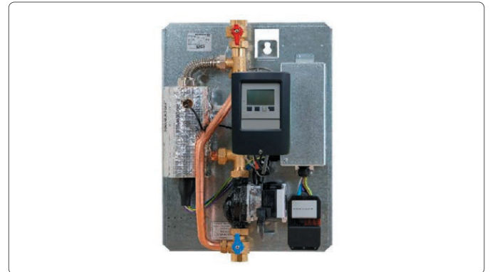
tubra®-eTherm C 3/C 9 3 kW or 9 kW electric boiler with target temperature control and a reheating thermostat for use as an external buffer tank charger powered by electricity. Can be used as a 3 kW or 9 kW Power-to-Heat hydraulic module for external power electronics such as Fronius Ohmpilot, my-PV AC: Thor, Elios4You, SMA Sunny Home Manager, and others. WPO22000 tubra eTherm C 3 3 kW WPO22030 tubra eTherm C 9 9 kW
