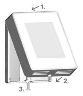
Refit the base and fasten with screw. Switch on the mains voltage and put Symondo Controller into operation.
